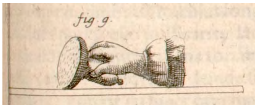
Figure 26: Diagram shows a lens-blank fixed using pitch or rosin to a short wooden or stone handle called a mollette. The tool was important in manual work to hold the lens-blank while shaping it on the form; and hold it while pressing down to be polished. However, the short handle and the wide distribution of force over the surface of the glass could lead to a rocking of the blank as it was guided over the form, resulting in distortions of shape. 165 Johann Zahn, Oculus artificialis teledioptricus , Herbipoli: Sumptibus Quirini Heyl, 1685–6, 'Fundamentum III', 'Practico-Mechanicum Fabrica', 34, Iconismus V, fig. 9. © Whipple Library, Cambridge, STORE 43:17.
